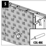
... glued together and glued together with the support construction. Apply the adhesive to the plate edges as an uninterrupted strand.
