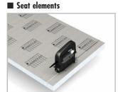
Cut two elements for the seat (top element = niche width x seat depth x 50 mm, bottom element = niche width -100 mm x seatdepth -50 mm x 50 mm) from ELEMENT-EL (Baby) 50.
