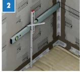
Mark the seat height (take into consideration thickness of the surface) and top edges of the support strips (= seat height -thickness of the surface -50 mm) on the three surrounding walls of the niche.
