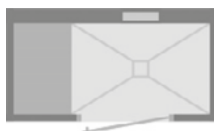
CAB-R 1780/950 R.LG * door DIN right / bench seat left of the door / installation wall opposite the door
