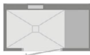
CAB-R 1780/950 R.RG * door DIN right / bench seat right of the door / installation wall opposite the door
