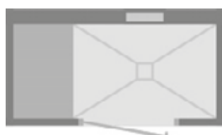
CAB-R 1780/950 L.LG * door DIN left / bench seat left of the door / installation wall opposite the door
